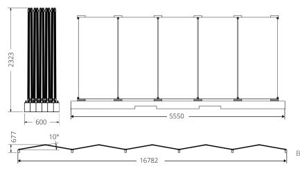
MAV model 5BAU-MAV-5P5B-16S-JAM72S10 390-410/PR Module Configuration 40 modules per MAV, 5 wide x 8 long Module Dimensions  $40 (H) \times 996 (W) \times 2015 (L) mm$ Packed Dimensions 5550 (W) x 2323 (H) x 600 (L) mm Packing Configuration 2 MAV units per 20' HQ container Deployed Dimensions 5550 (W) x 677 (H) x 16782 (L) mm Deployment Type Telehandler or forklift
